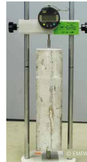
The increase in volume due to the strain resulting from ASR becomes perceptible by measurement of a change in length of test specimens. Ordinarily the specimens are stored under intensified conditions (temperature, humidity, applied load) in order to accelerate the reaction.
