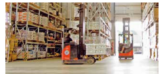
Industrial flooring surfaces also experience strong abrasion due to constantly rolling and striking loads in the same places. Hard concrete coatings and special dispersants can enhance the flooring grip and minimize wear.
