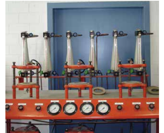
Water absorption of concrete under pressure measures the maximum water penetration in mm after a defined time with a specified pressure. (24 hours with 5 bar according EN12390-8)
