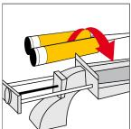
When the work is interrupted the static mixer nozzle can remain on the cartridge after the gun pressure has been released. If the resin has hardened in the nozzle when work is resumed, a new nozzle must be attached.
