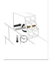
9. Do not load or move the anchor during the hardening time.
