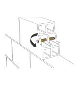
8. IMPORTANT The anchor must be placed within the open time. Insert the anchor with a rotary motion into the filled perforated sleeve. Use the appropriate steel rod size. Note Some adhesive must come out of the hole.
